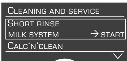
The milk system **10** can be pre-cleaned automatically.
