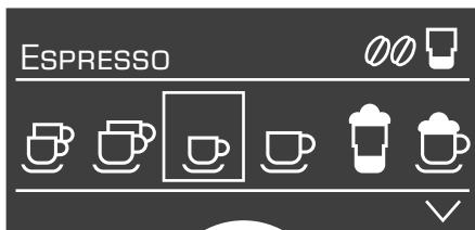
The status line **5a** in the display **5** shows the name of the type of drink, along with the strength setting, e.g.  $\textcircled{0}$  and per-cup quantity, e.g.  $\textcircled{1}$ . The selection line **5b** shows symbols for drink selection.
