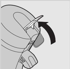
**3 Move the lever upwards to release the lid.**
