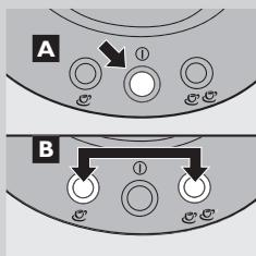
**9** Press the on/off button ① and subsequently press the 1-cup button ② and the 2-cup button ③ briefly at the same time.
